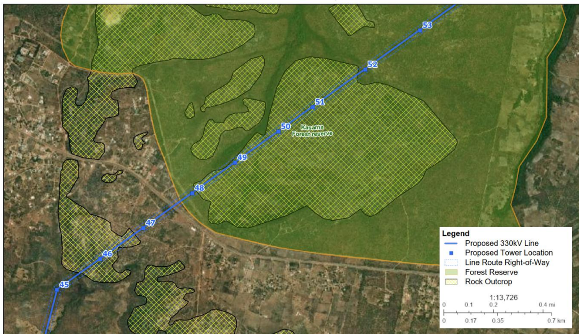
Figure 3-1 Pylon Location in Rock Outcrops
